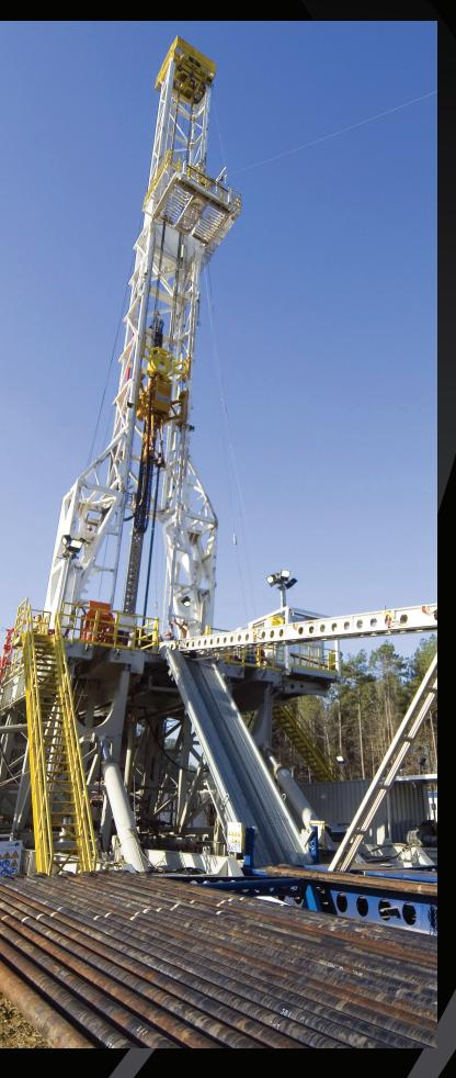
The Automated Power Catwalk is simple to use and extremely robust. It combines innovative engineering and proven manufacturing techniques to deliver a product that is designed for the optimum in personnel safety, virtually eliminating the need for manual handling of tubulars.
