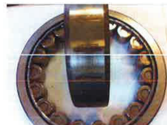
Figure 24: Surface marks (false brinelling)
