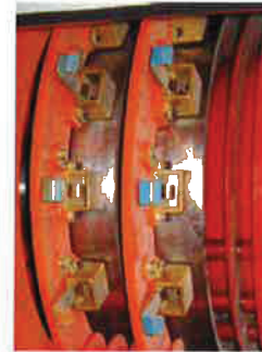
Figure 4: Brushes removed from the brush holder
