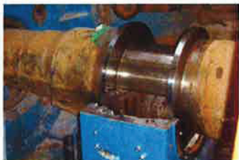
Figure 27: Corrosion on the shaft
