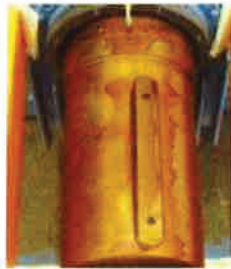
Figure 2: Anticorrosive product on machined parts
