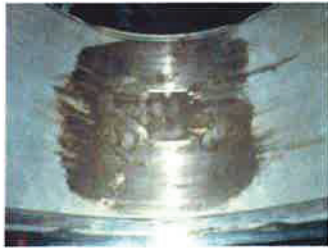
Figure 25: Marks on the bearing shell
