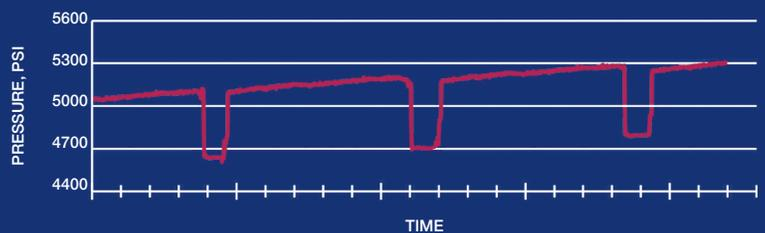
**BHP Response During Connections Utilizing Non Stop Driller**
