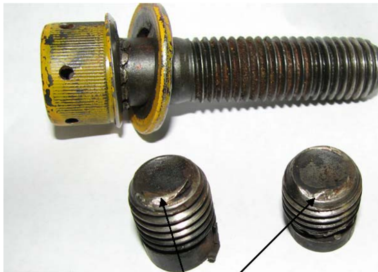
Signs of bolts bottoming out in the tapped holes of the Main Housing and/or the Frame Base Legs
