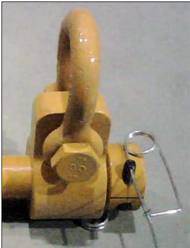
Figure 2: New-style torque track lifting bar
