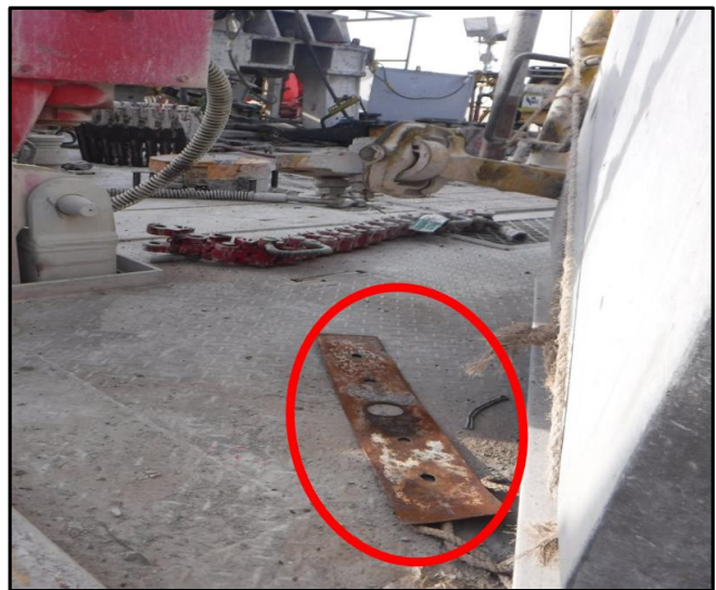
Figure 1: Bolts heads from torque restraint sheared, causing liner and metal shims to fall to the rig floor
