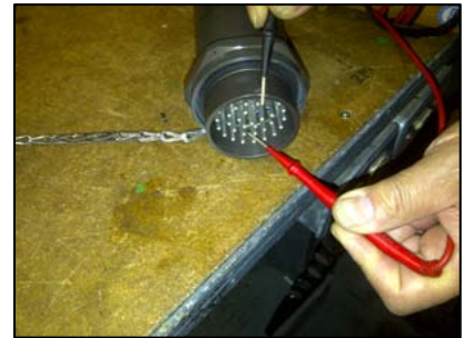
Figure 5: Place a DVM leads across Pin 3 and filed end of cable
