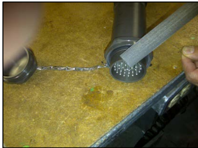
Figure 3: Filing the outer case of the Pyle National sheet
